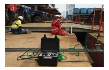
The MOSS multi channel indicator is a practical, robust, portable measurement solution solving your autonomous monitoring, logging surveying needs.
