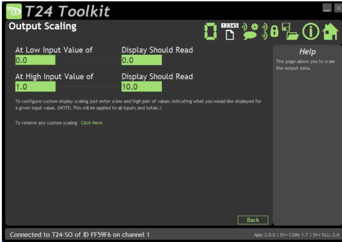
This page allows effective conversion between units. i.e. Although all devices supplying data are configured in Kg you can get a printed output in Lbs.
