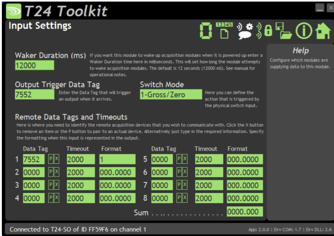
Here you can set the action to take when the switch contacts are closed, set the Data Tag that will trigger an output and also set the Data Tags of the data used as the inputs along with how the data is formatted.
