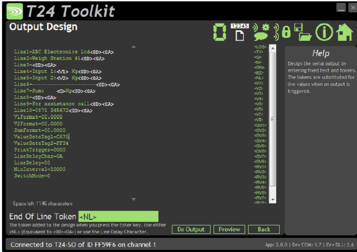
This is where you define the actual output based on free text and tokens. Tokens are special codes contained within angled brackets <token> which have special meanings and are converted to actual values once an output is triggered. See list of tokens at the bottom of this section.
