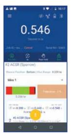
Screen showing slider graph and tolerance setting.
