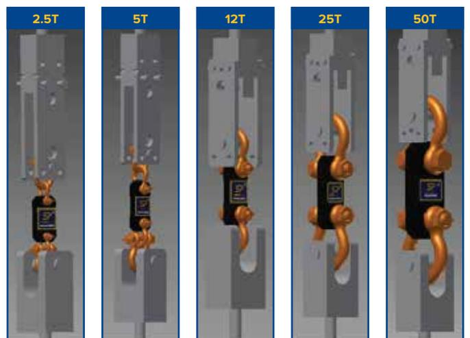
Developed to assist our global network of Straightpoint partners this test machine has been designed to allow local calibration of our range of Loadlink, shackle and crane weigher products up to 55 tonnes capacity.
