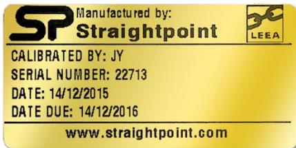
**Data Tag** – This is a unique code for the loadcell, and is always the last four digits of the loadcell serial number. This is 2713 in the above image.
