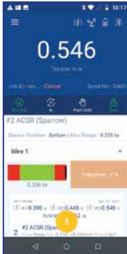
Screen showing slider graph and tolerance setting.
